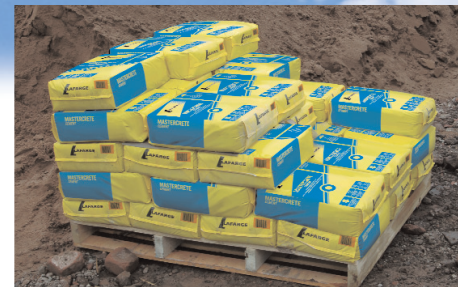
Undamaged plastic packaging on building site.
